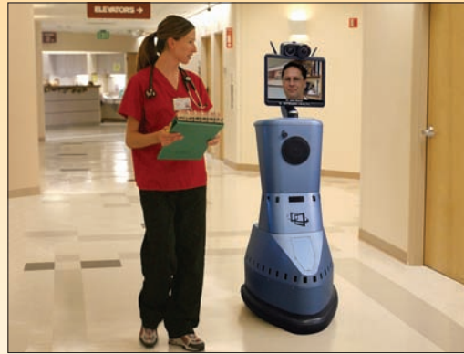
The Remote Presence Robot (RP-7) from InTouch Health is a mobile telemedicine unit that connects physicians and specialists with patients and other doctors in real time through computers equipped with cameras and microphones.
